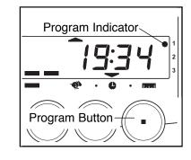
manual mode, press the program button until the program indicator disappears. The programs will be selected in the following order: program 1 (Interval), program 2 (Aerobic), program 3 (Fat Burn), manual mode.
